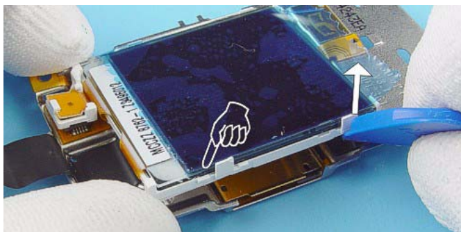
34.) Place the SRT-6 between LCD and the LCD Can as shown in the picture and lever out the LCD carefully.
