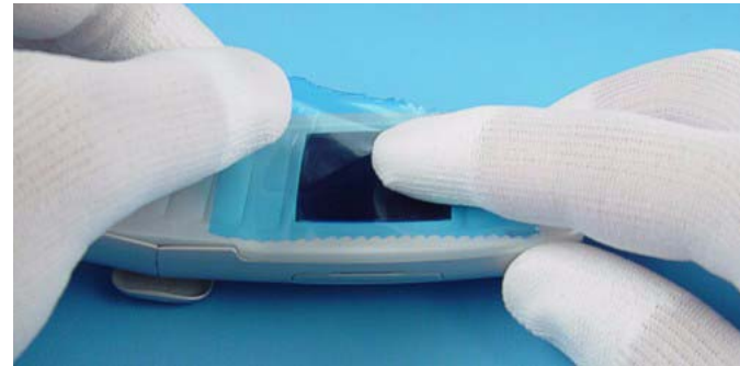
2.) Open the unit and protect the Window with a plastic film.
