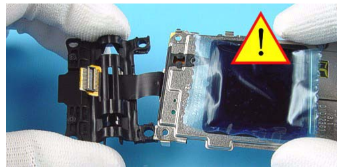
27.) Take care not to damage the Flex Connector when removing the Plastic Hinge.
