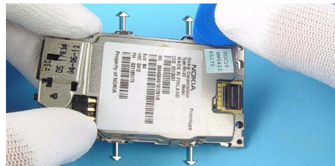
35.) Release the four springs of Key Dome Shield.
