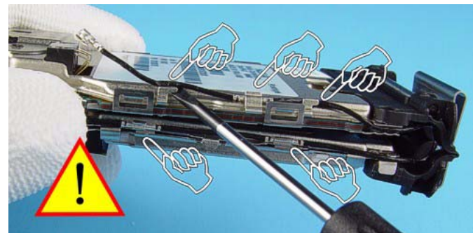
19.) Note the exactly position when laying the Coax Cable during assembly.
