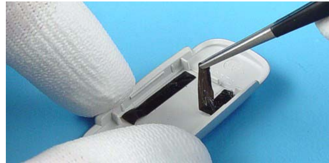
4.) Now, remove the Backplate adhesive. If necessary clean the Backplate and the Hinge Spring before attaching using new Backplate Adhesives.
