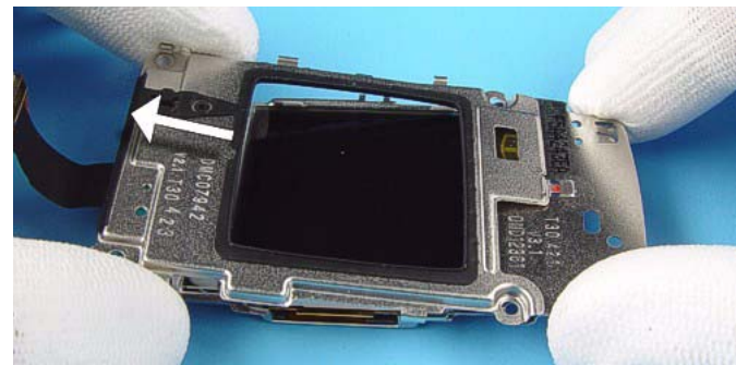
31.) Separate the C2-Cover from LCD CAN Assy.
