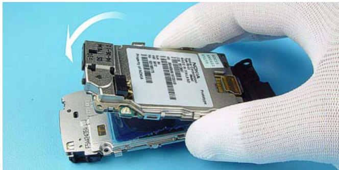
22.) Put the Lower Block on the Upper Block as shown in the Picture.
